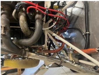
Right: note crack in old pipe found during 100 hr inspection. Pencil to show the scale.
