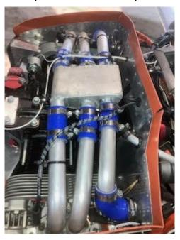
Below Left: Left Cyl bank Fuel Injectors (2) above Aluminum Rocker Cover. Right: Fuel Injection pump with 4 outputs (1 per cylinder, and input on Left.)
