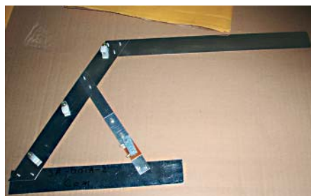
Aerials: mounted vertically inside each fibreglass winglet is this VHF aerial. Aluminium foil connects it to the carbon fibre wing structure which serves as a massive ground plane.
