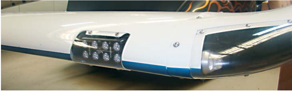
LED landing lights and strobes use less current, always a consideration with this all-electric aeroplane.
