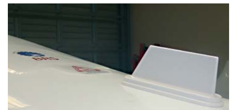
With the transponder aerial in the aft keel, the only external antenna is the ELT, just aft of the ballistic recovery chute.
