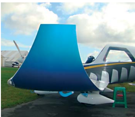
Aerials: mounted vertically inside each fibreglass winglet is this VHF aerial. Aluminium foil connects it to the carbon fibre wing structure which serves as a massive ground plane.
