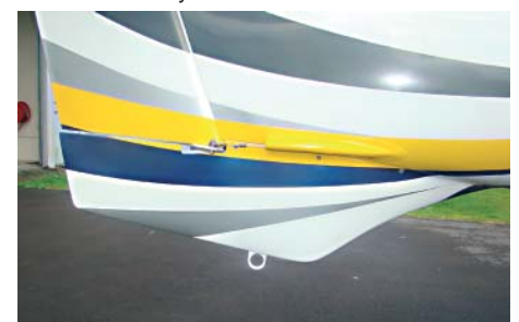
With the transponder aerial in the aft keel, the only external antenna is the ELT, just aft of the ballistic recovery chute.
