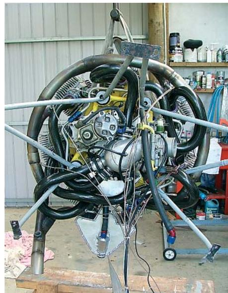
changing baffles and cowling to aid cooling. Hopefully these changes will have the desired effect.
