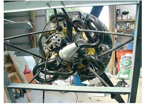
Each induction pipe is the same length but a different shape to fit around accessories and mount frame tubes.
