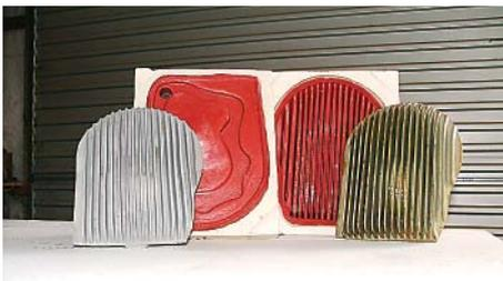
The heads were a simpler process, made difficult by my using tube silicon to seal up cracks in a very simple mould. To my disgust methyl ethyl ketone (MEK), a solvent vapour given off from tube silicon, completely stuffed the curing of the two-pot silicon. I finished up with \$200 worth of goey, partly cured, stick-to-everything silicon to clean up. Needless to say this didn't make it to the offering shelf as it would have made things more than a bit sticky up there.
