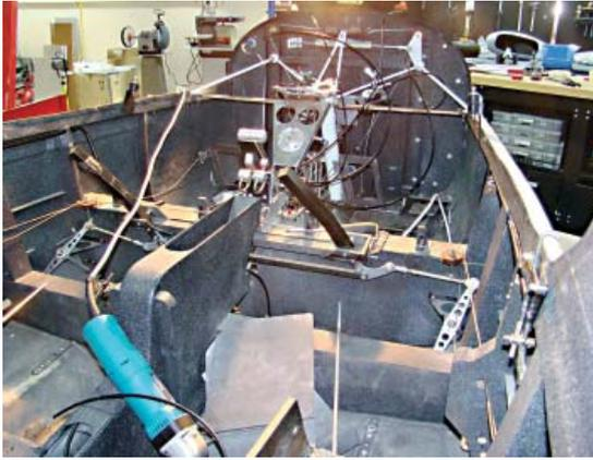
Structure and systems start to go together in the forward part of the cabin. The nose leg is aft of the firewall.
