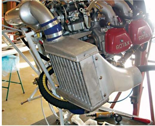
This Rotax 914 is equipped with intercooler for its turbocharger.
