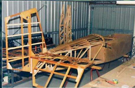
large model aeroplane and this is what it turned out to be, but instead of balsa wood I used Douglas fir, Sitka spruce and Hoop pine. Laying out and gluing up the fuselage framework on my 16 by 4 foot workbench went ahead quite quickly with no problems, and soon I had two sides of the fuselage completed.
